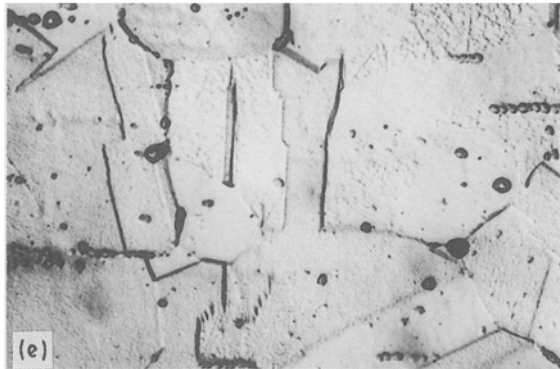
Figure 7 Microstructure after EPR and 10% OAE tests in specimens either strained at \dot{\epsilon} = 4.16 \times 10^{-4} \text{ s}^{-1} or isothermally treated at 823 K. (a)–(c), EPR test, (d) and (e), 10% OAE test. (a), \epsilon = 0.072 t = 3.9 ks, (b) and (d), \epsilon = 0.22 t = 4.2 ks, (c) and (e), isothermal treated t = 3.6 ks.
